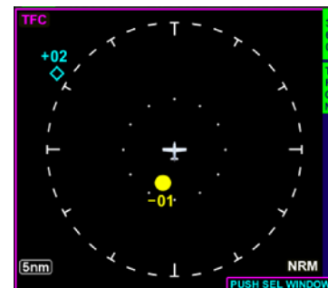
Figure 2-3 Dedicated Traffic Display
