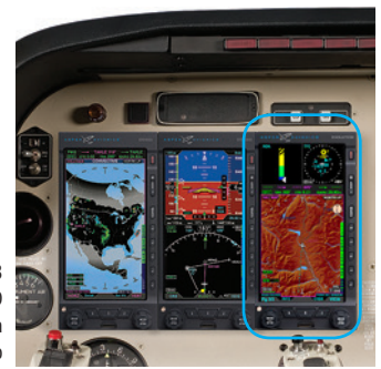
Figure 5-113 The EFD1000 MAX MFD is on the Right of a Three-Display Setup
