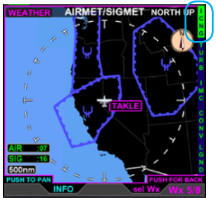
Figure 5-81 METAR Product VIEW Showing Icing AIRMET
