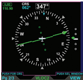
Figure 5-112 Secondary HSI Displaying the VDI
