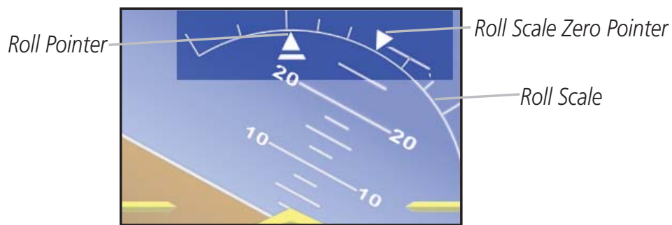
G500 Attitude Indicator with a Ground Pointer Configuration in a Left Turn
